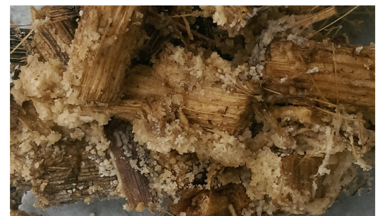
Used filter material impregnated with ammonium sulfate that can be used as fertilizer
